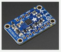
Inertial Measurement Unit
