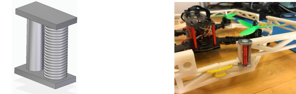
Figure 7. A 3D model of the electro-permanent magnet housing showing a pair of AlNiCo magnets, one encased in a coil.
